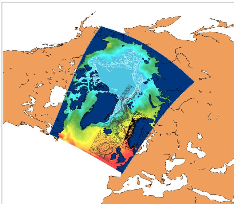
*Figure 1: Nested operational hydrodynamical model system at MET Norway. Grid spacings: outer domain 20 km; intermediate domain 4 km; inner domain 800 m. Outer model gets open boundary conditions from UK Met Office's FOAM system.*
